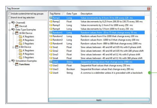
In the right-hand pane, select Click to add IoT items. In the Tag Browser, select the items you would like to read through the gateway. This guide uses data generated from the Simulation driver, including Ramp1, Random1, and User1 from the "Simulation Examples. Functions" channel and device.
