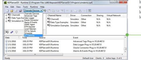
In the KEPServerEX Configuration window, use the drop-down menu located in the toolbar to select the IoT Gateway.
