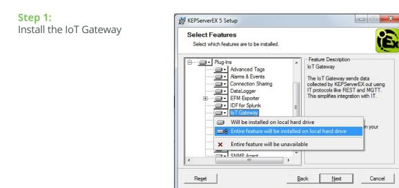
The IoT Gateway is installed as an advanced plug-in to the KEPServerEX connectivity platform. During the -KEPServerEX installation, expand the Plug-Ins option to locate the IoT Gateway in the Select Features dialog. Then, select Entire feature will be installed on local hard drive and complete the install.
