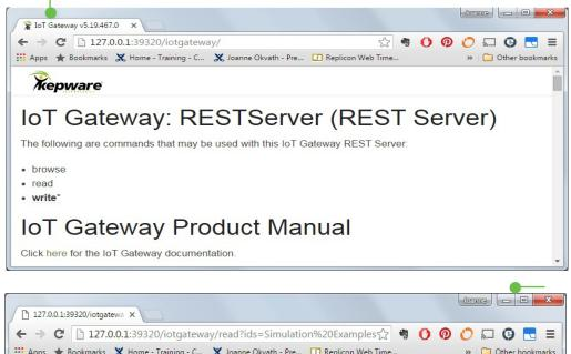
To perform a read, enter "http://127.0.0.1:39320/iotgateway/ read?ids=Simulation%20Examples. Functions.User1" into the address bar and then press **Enter**. If you used something besides the Simulation Examples item, enter your tag item in the format of "Channel.Device. Tag" after the "read?ids=" in the URL.
